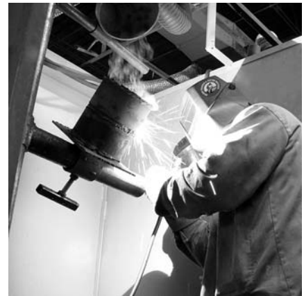
Student practicing a weld on pipe
